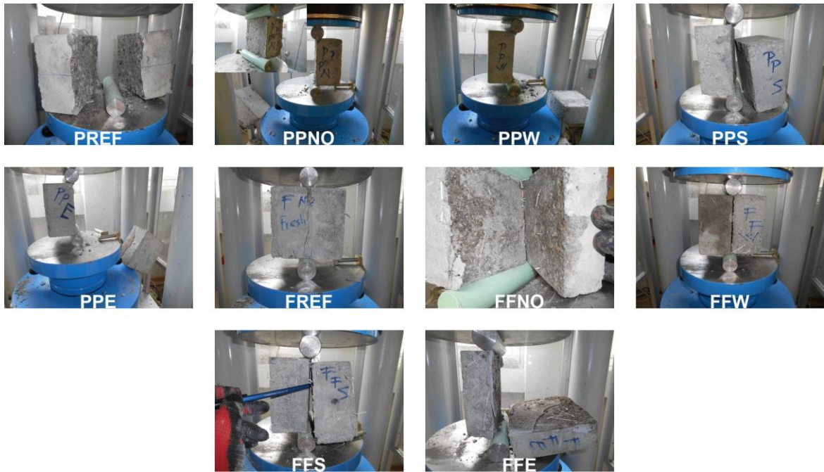
Figure 75. Failure modes observed in the split prism tests conducted on jointed RCC
