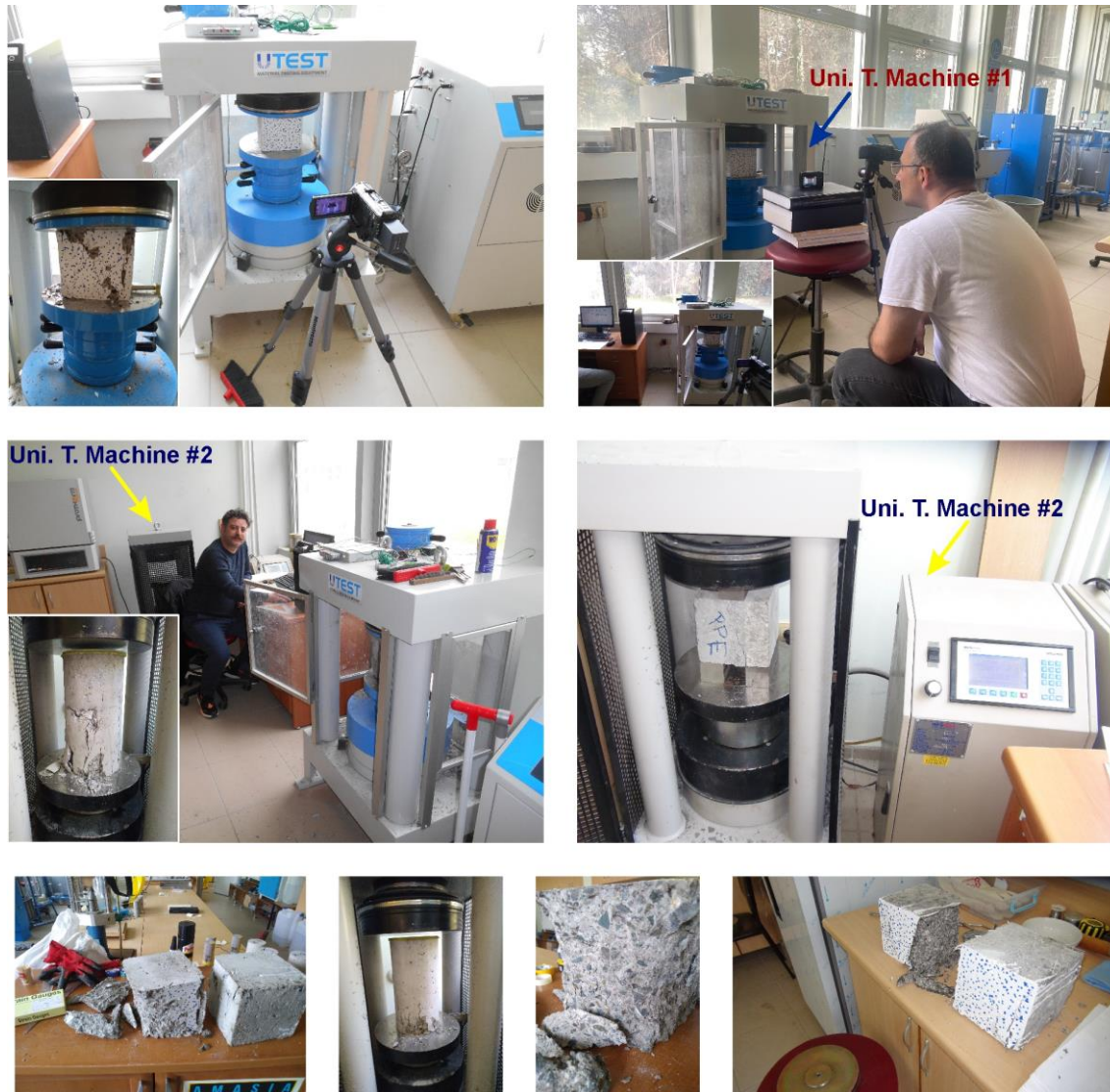
Figure 50. The test setup of a universal testing machine for measuring the compressive strength of RCC samples
