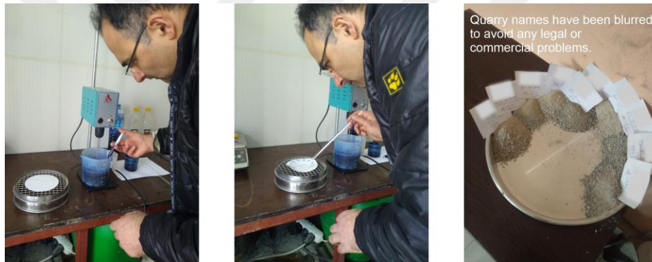
Figure 40. Defining the MBI level of the fines in sand
