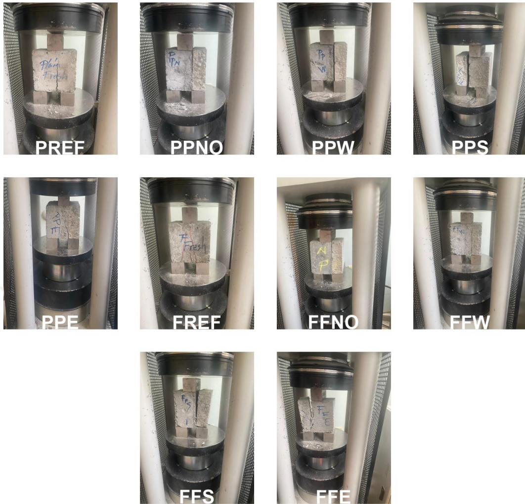
Figure 79. Failure modes observed in the bi-surface shear tests conducted on jointed RCC
