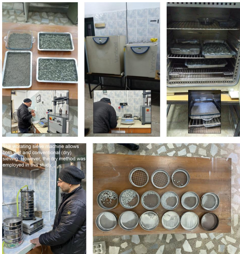
Figure 41. Aggregate samples used in the production of fresh RCC
