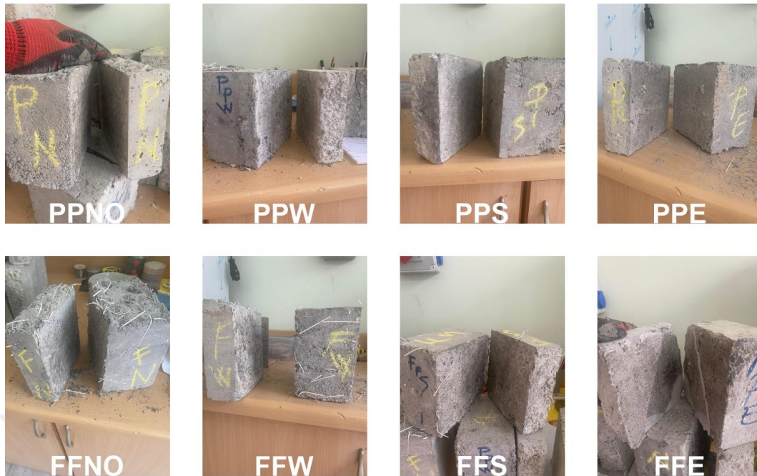
Figure 80. Fracture surfaces of the bonded specimens in a bi-surface shear test
