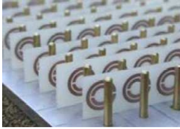
Figure 3.4: First metamaterial comprised of metallic rods and circular split rings.
