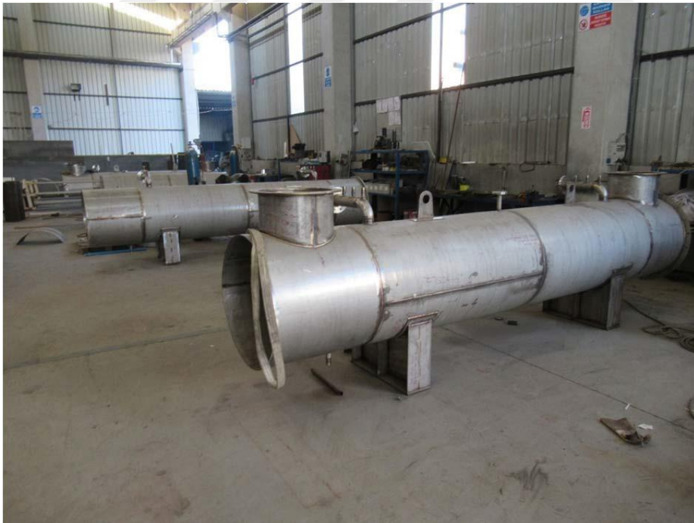
Figure 4-8. Manufacturing of heat exchanger.
