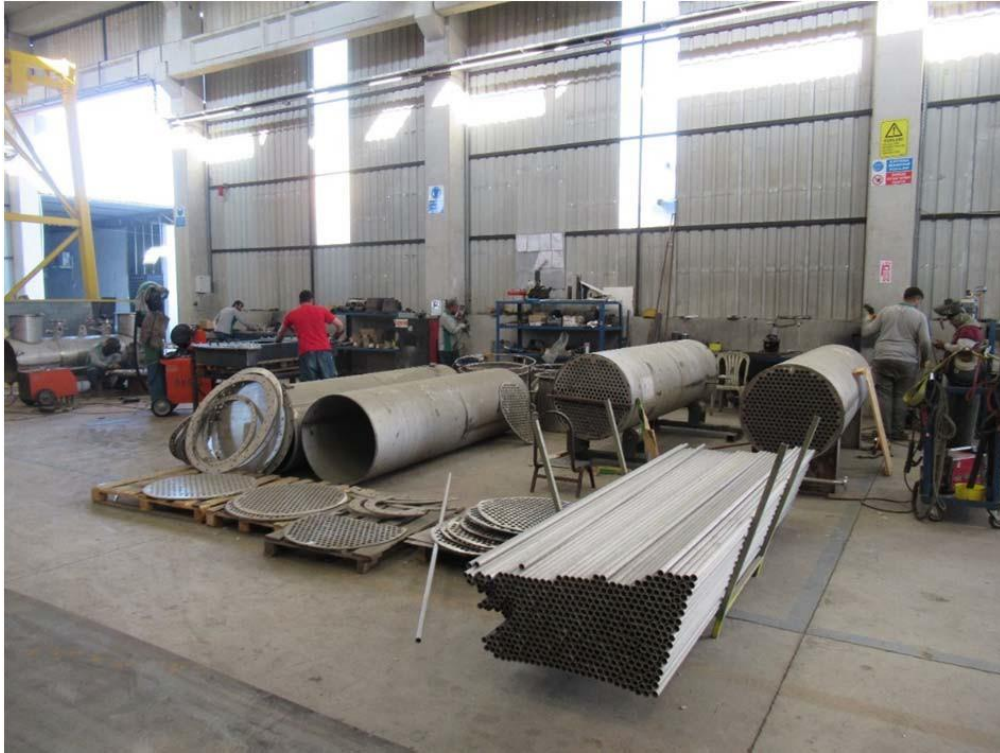
Figure 4-7. Manufacturing of heat exchanger.
