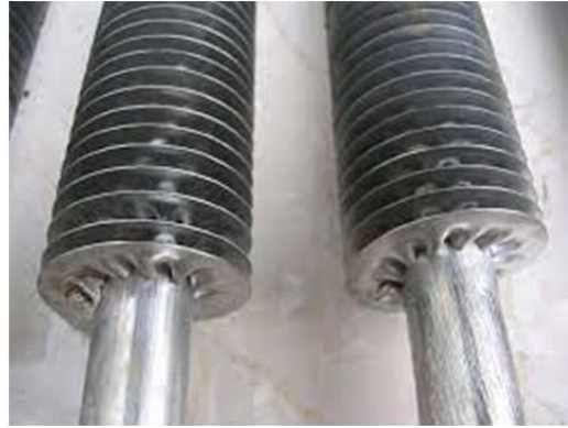
Figure 2-12. Finned Tube for Heat Exchanger.
