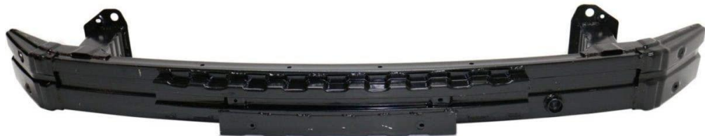
Figure 1.4: The bumper reinforcement bar [8].
