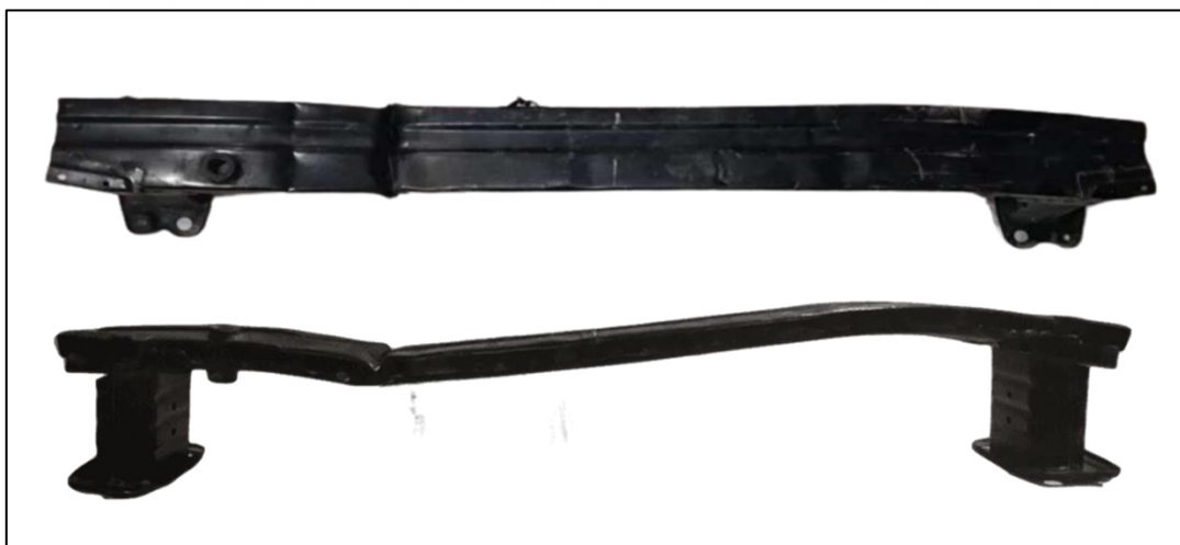
Figure 4.15: The picture shows the shape of the original bumper of the KIA Optima 2019 after being deformed
