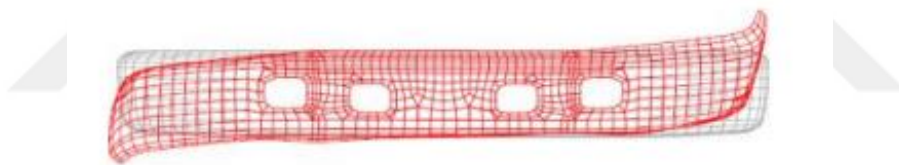
Figure 3.20: FEA model of a supporting brackets and front bumper.
