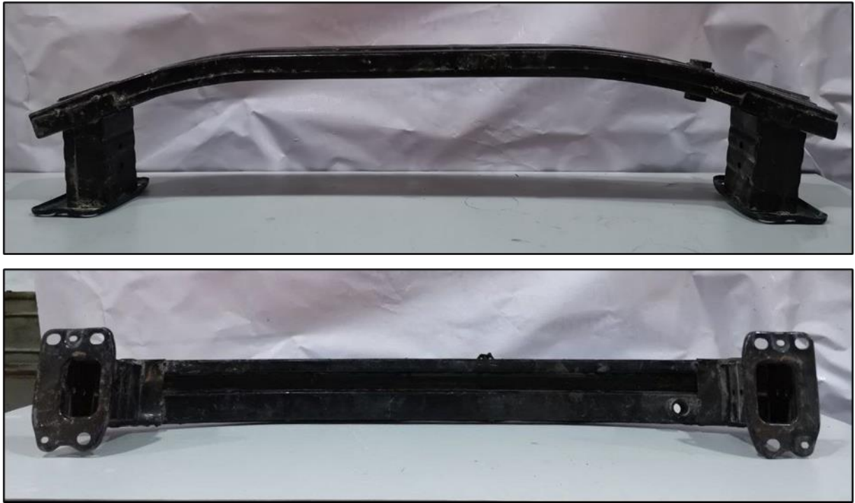
Figure 3.23: A Full-Scale Size of the Bumper Beam Specimen.
