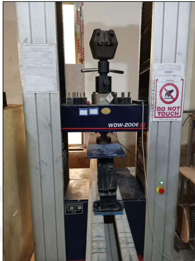
Figure 3.22: Electronic Universal Testing Machine WDW-200E.
