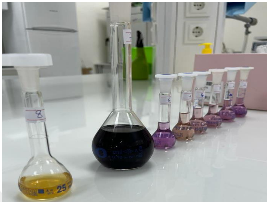
Figure 4.17 Reaction of the Ganoderma lucidum extract obtained by Soxhlet extraction at different concentrations with DPPH solution of 166.60, 499.80, 833.00, 1166.20, 1499.40, 1999.20, 2499.00 and 3332.00 \mu\text{g/mL}
