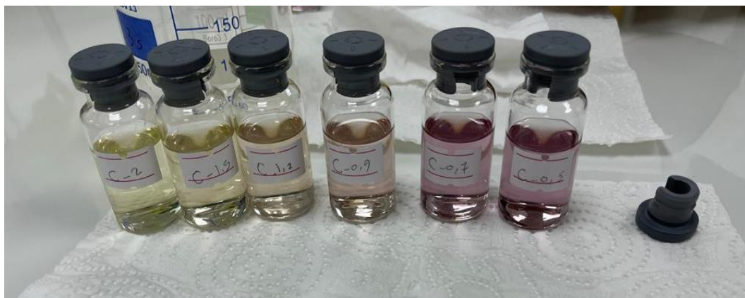
Figure 4.20 Reaction of the Ganoderma lucidum extract obtained by sonication extraction at different concentrations with DPPH solution of 166.60, 499.80, 833.00, 1166.20, 1499.40, 1999.20, 2499.00 and 3332.00 \mu\text{g/mL}
