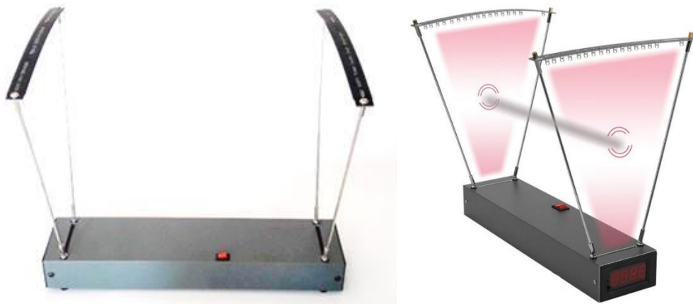
Figure 3.4: The velocimeter device for measuring penetration speed and the exit velocity.
