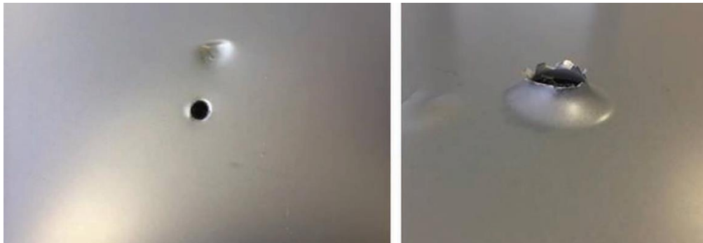
Figure 4.1: The 36mm rifle projectile orthogonal impact [32]
