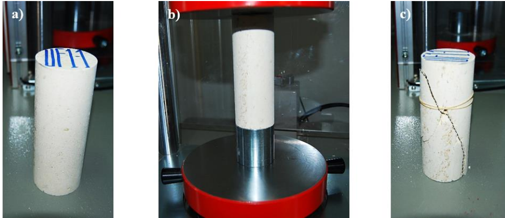
Figure 2.15. Bayburt tuff specimen subjected to UCS and cyclic loading test
