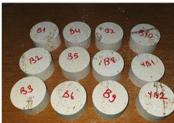
Figure 2.11. BTS test for Bayburt tuff specimens
