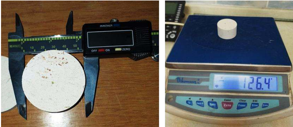
Figure 2.3. Physical measurements from Bayburt tuff specimens
