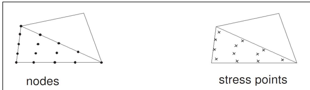
Figure 2.4 Example of nodes and stress points positions in mesh element [34]
