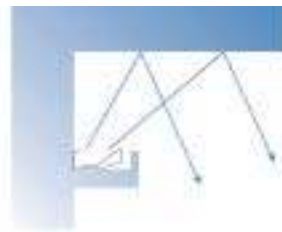
Figure 2.10: Vertical section of a cove lighting system
