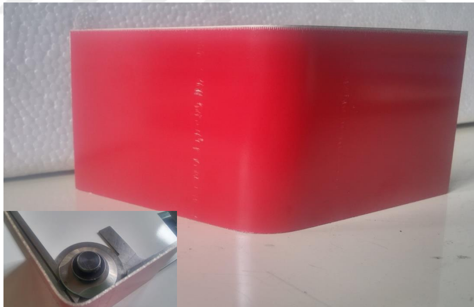
Figure 6.1 Cold Bent Specimens with Angle of 90^{\circ}
