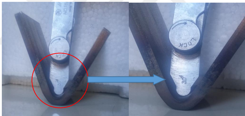
Figure 6.27 Radius measurement of 1.4003 After Bending Operation
