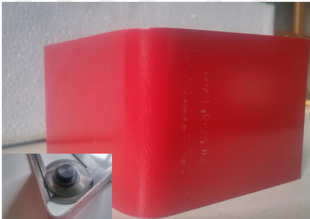
Figure 6.3 Cold Bent Specimen with Angle of 75°
