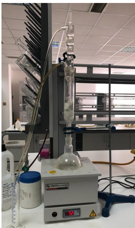
Figure 3.4: Soxhlet Extraction of Pistacia lentiscus L.
