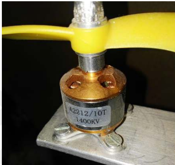
Figure 3.2 UAV Brushless Motor A2212/10 1400KV
