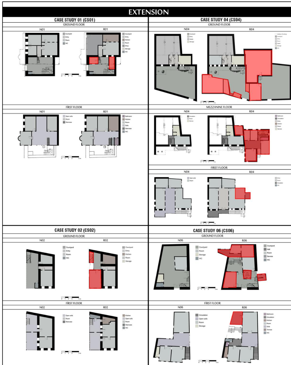
Figure 3. 20. The extended areas shown on the floor plans of case studies CS01, CS02, CS04 and CS06, are indicative of the existence of the flexible design parameter called 'Extension'
