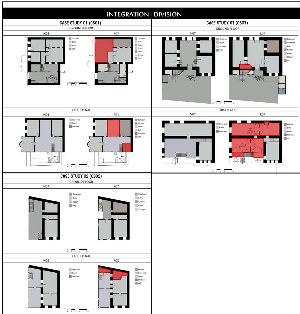
Figure 3. 19. The integrated-divided areas shown on the floor plans of case studies CS01, CS02 and CS07, are indicative of the existence of the flexible design parameter called 'Integration/division'
