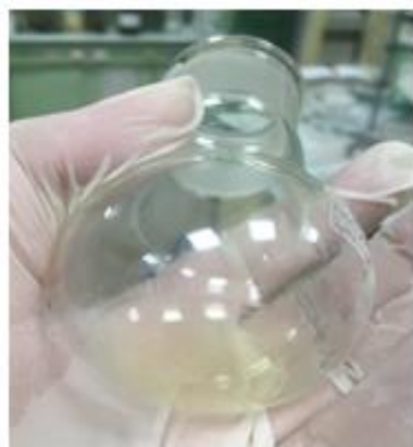
Figure 4.13. Smooth and homogenous SPE film showing no untrapped SPE spot
