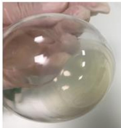
Figure 4.14. Thin film showing huge untrapped SPE spot (circle)
