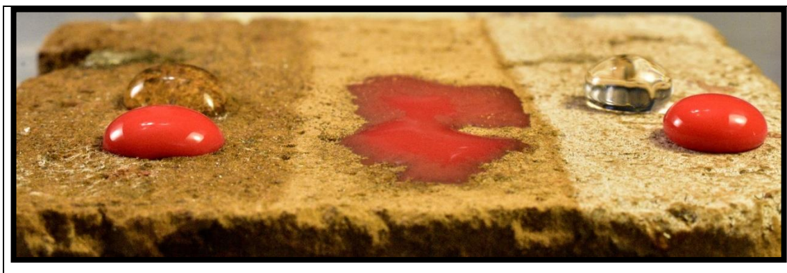
Figure 3.23. SOL2 (left) coated, uncoated (middle) and SOL4 (right) coated Ahlat stone with red dye and water drops
