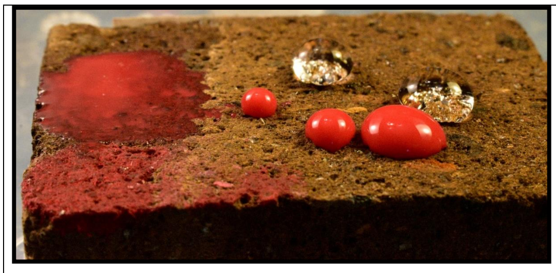
Figure 3.25. SOL5 coated (right) and uncoated (left) Ahlat stone with dye and water drops
