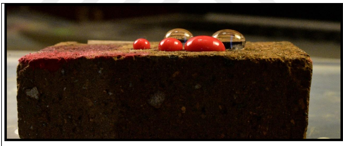
Figure 3.26. SOL5 coated (right) and uncoated (left) Ahlat stone with dye and water drops
