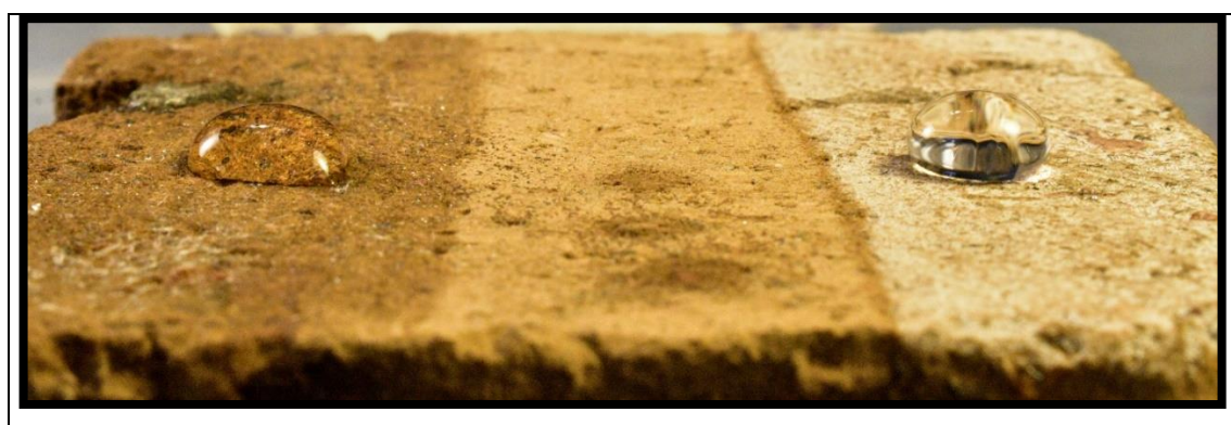
Figure 3.24. SOL2 (left) coated, uncoated (middle) and SOL4 (right) coated Ahlat stone with water drops
