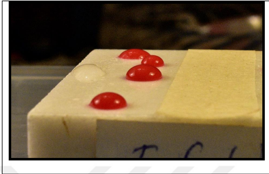
Figure 3.37. SOL 5 coated (left side) Marmara Marble exposed dye and water
