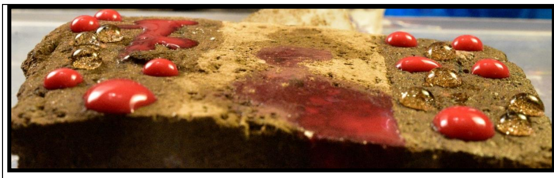
Figure 3.21. SOL1 (left) coated, uncoated (middle) and SOL3(right) coated Ahlat stone with red dye and water drops
