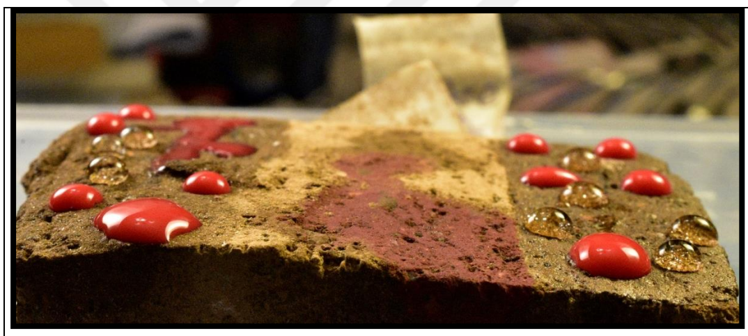
Figure 3.22. SOL1 (left) coated, uncoated part (middle) and SOL3(right) coated Ahlat stone with red dye and water drops after 20 seconds
