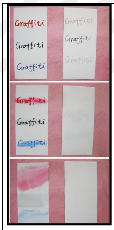
Figure 1.4. Comparison of anti-graffiti properties between RPU (left) coating and AGPU (right) coating [65]
