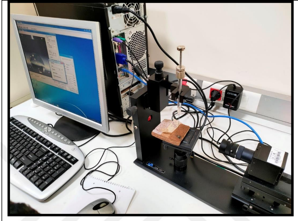
Figure 2.2. Goniometer measurements with coated Ahlat stone
