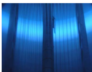
Figure 3.3. Textile fibers in the plasma coating plant [43]
