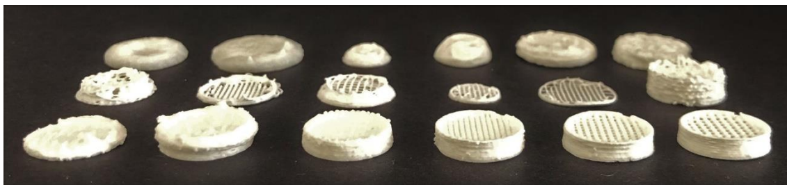
Figure 5.4. Image of the tablets resulting from the gradual experimental optimization of paste/ink and printing settings (side view)
