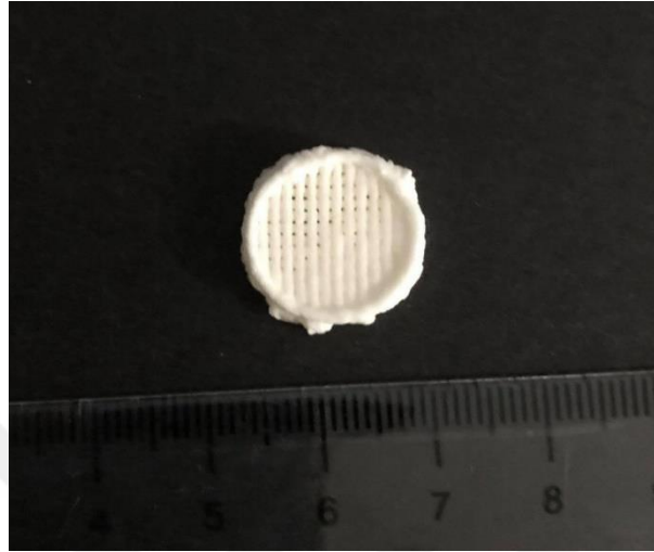
Figure 5.2. Inconsistent strand diameter attributed to poor hydration of paste
