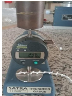
Figure 2.9 The rope diameter evaluation via thickness gauge
