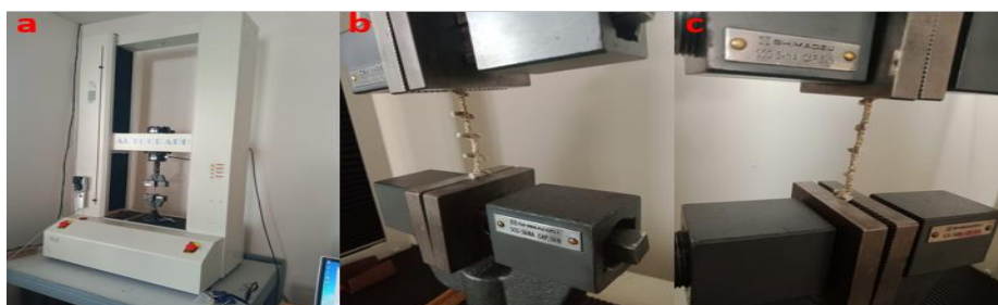
Figure 2.8 a) Tensile strength test device, b) Single rope test sample that placed between holder clamps
