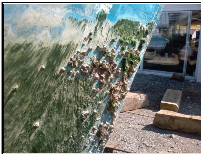
Figure 1.1 Biofouling on the vessel hull (Photo: Zeynelabidin KARABAY).
