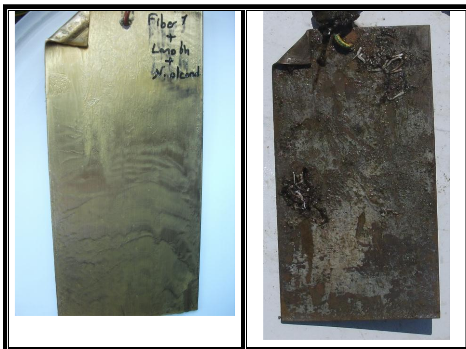
Figure 3.37 The metallic plates (Lanolin based material, Fiber 1 and N.oleander extract) exposed in Zeytinburnu coast 2 months immersion, left: before immersion, right: after 2 months.
