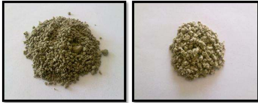
Figure 2.1 The commercial fibres which provides from Lapinus Company in Netherland: (left) Rockforce MS730-Roxul 1000, (right) Rockforce MS675-Roxul 1000.
