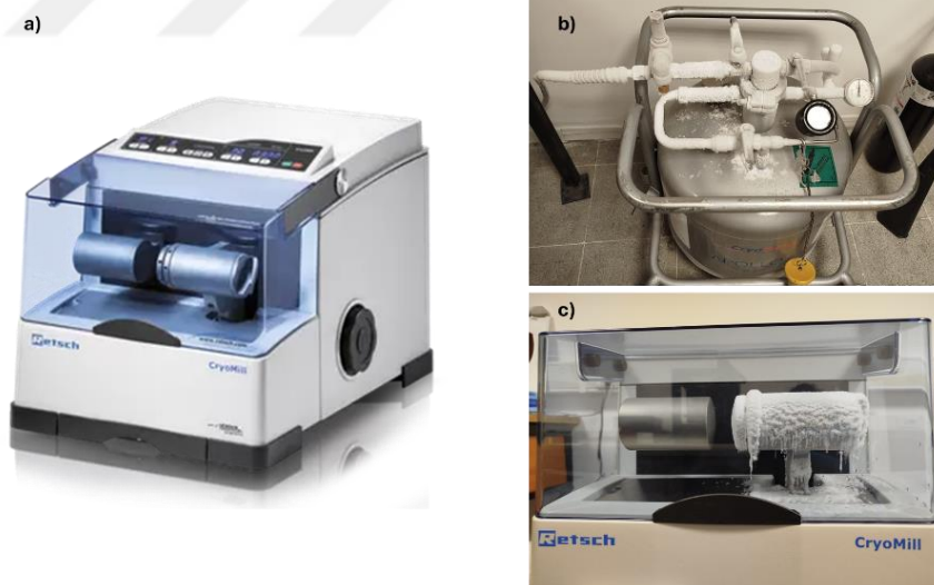
Figure 8 : The images of a) cryomill instrument (adapted from [54] ), b) liq. \text{N}_2 tank connected to instrument, c) frozen jar holder with the jar inside.
