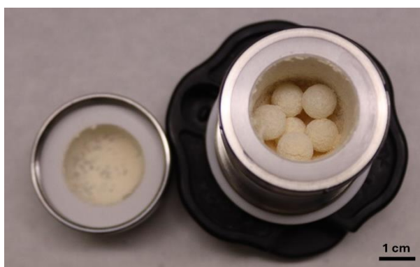
Figure 10 : A typical view of the milling materials and the reaction mixture after milling. The mixture was collected carefully and completely from the jar and milling balls.
