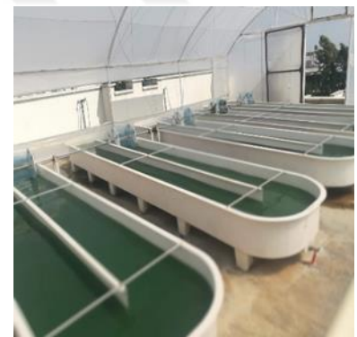
Figure 2.3. (A) Raceway tank for Spirulina cultivation. (B) Image Algal Biotechnology culture unit outdoor of Çukurova University in Adana, Turkey(original).
