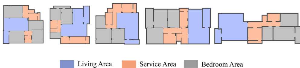
Figure 5.10: Functional Areas of Nilüfer Apartment (1967), Özen Apartment (1969), the 1970 Apartment (1970), Uğur Apartment (1973), Galip Bey Apartment (1977).
