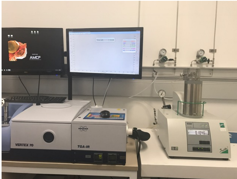
Figure 9.9: Conducting TGA Analysis on Polymers and Their Blend
