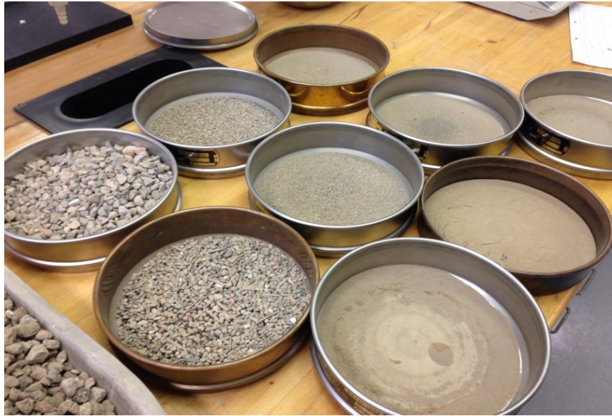
Figure 4.2: Aggregate Gradation by Particle Size Distribution Test
