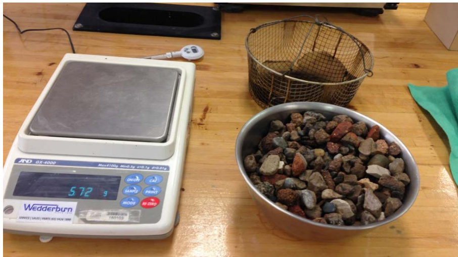
Figure 4.6: Conducting Particle Density and Water Absorption Test on Coarse Aggregates
