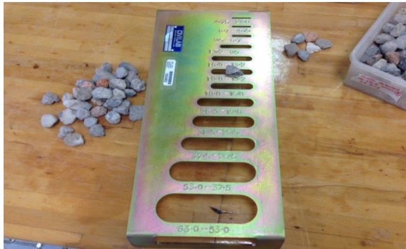
Figure 4.5: Conducting Flakiness Index Test for Coarse Aggregates
