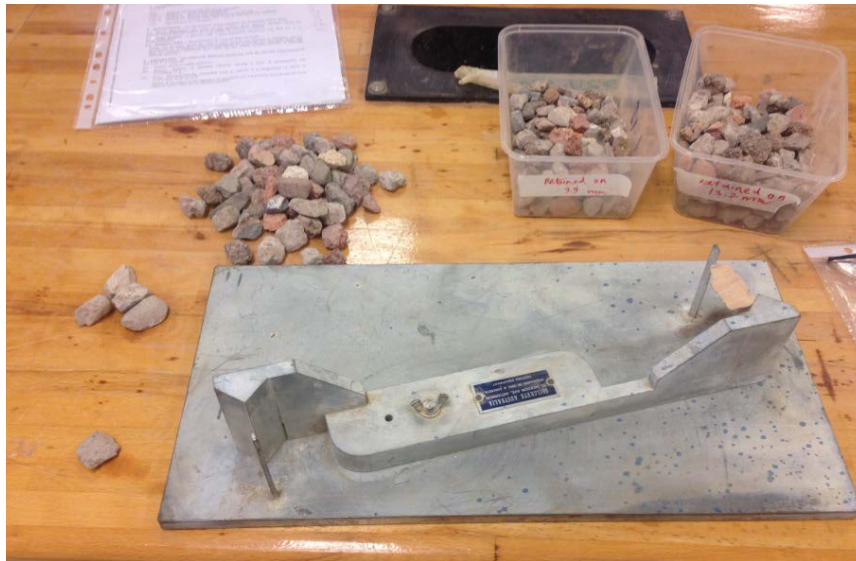
Figure 4.4: Classification of Coarse Aggregate Based on Particle Shape Test
