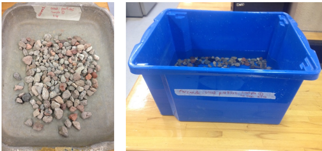
Figure 4.9: Conducting Weak Particle Test for Coarse Aggregates
