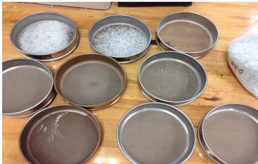
Figure 4.20: Glass Gradation by Particle Size Distribution Test
