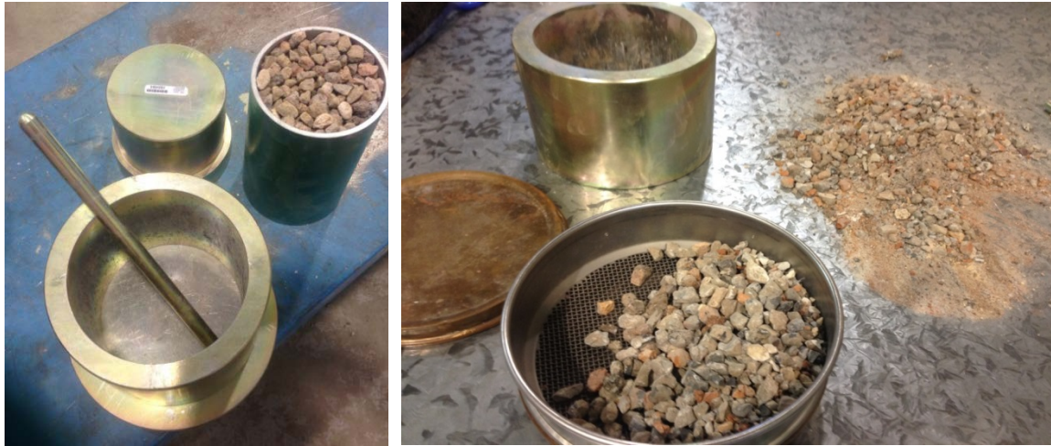
Figure 4.8: Conducting Crushing Value Test for Coarse Aggregates
