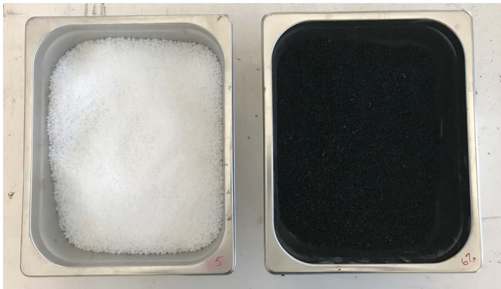
Figure 3.4: Used Binder Modifier Including HDPE, and Crumb Rubber (from left to right)
