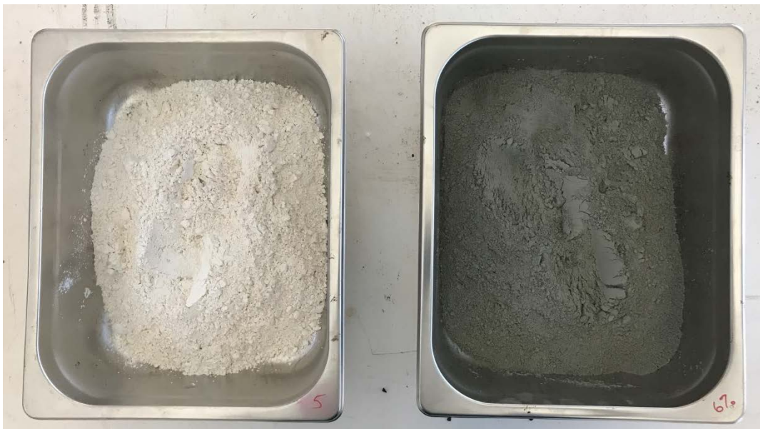
Figure 3.3: Used Filler Including Hydrated Lime, and Portland Cement (from left to right)
