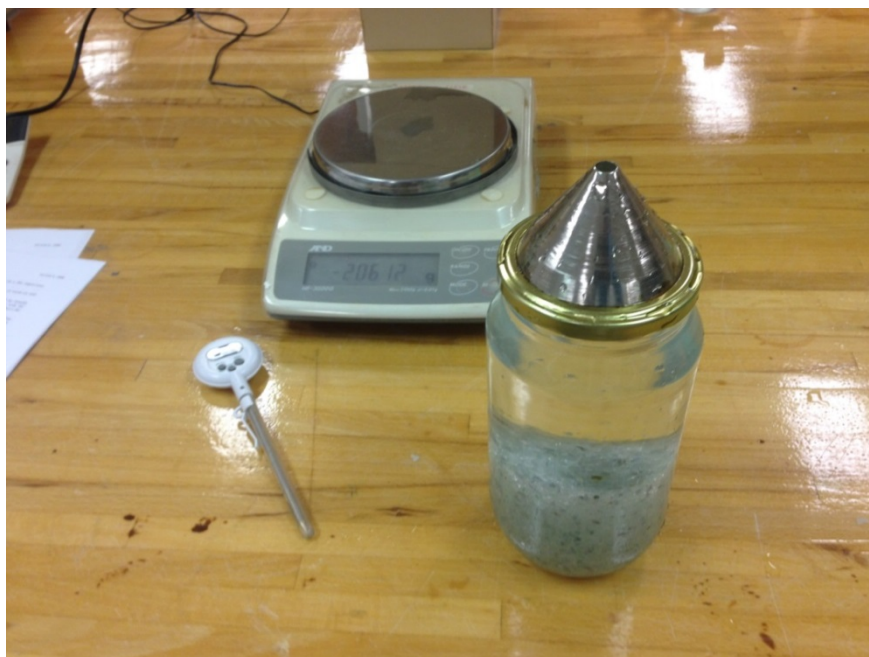
Figure 4.23: Conducting Particle Density and Water Absorption Tests on Glass
