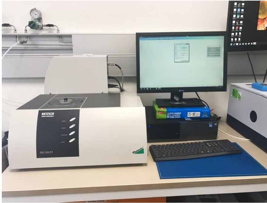
Figure 9.7: Conducting DSC Analysis on Polymers and Their Blend
