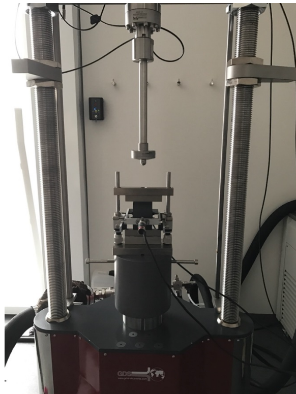
Figure 8.3: Resilient Modulus Test Conduction
