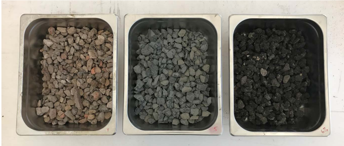
Figure 3.1: Used Coarse Aggregates Including RCA, Basalt, and RAP (from left to right)
