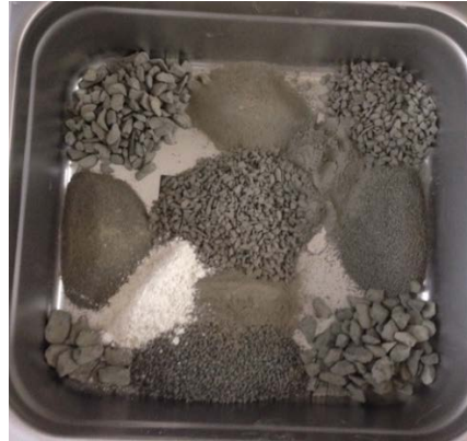
Aggregate and filler in Conventional Mixing Method
