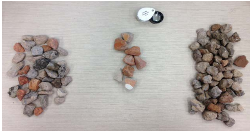
Figure 4.15: Classification of Recycled Construction Aggregate (RCA)
