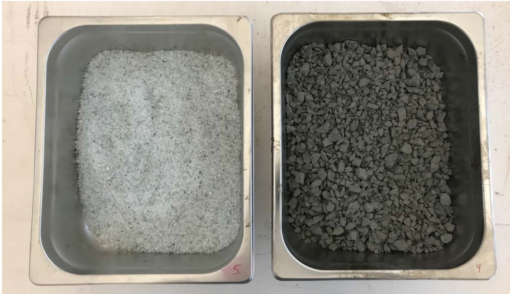
Figure 3.2: Used Fine Aggregates Including Basalt, and Recycled Glass (from left to right)
