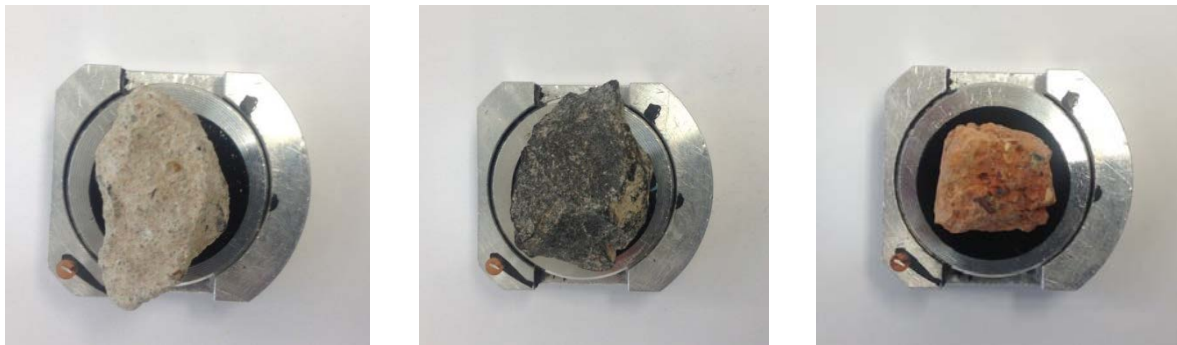
Figure 4.16: Studied Rocks from RCA Sample (a) Sedimentary, (b) Igneous, (c) Metamorphic
