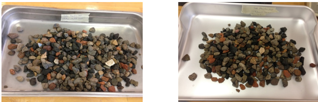
Figure 4.7: Particle Density and Water Absorption Test on Mix of Coarse Aggregates
