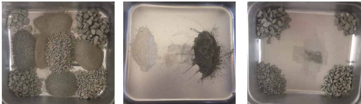
Aggregate and filler in New Mixing Methods (from left to right): Coarse, Filler, Fine
