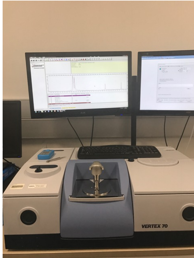
Figure 9.10: Conducting FTIR on Polymers and Their Blend
