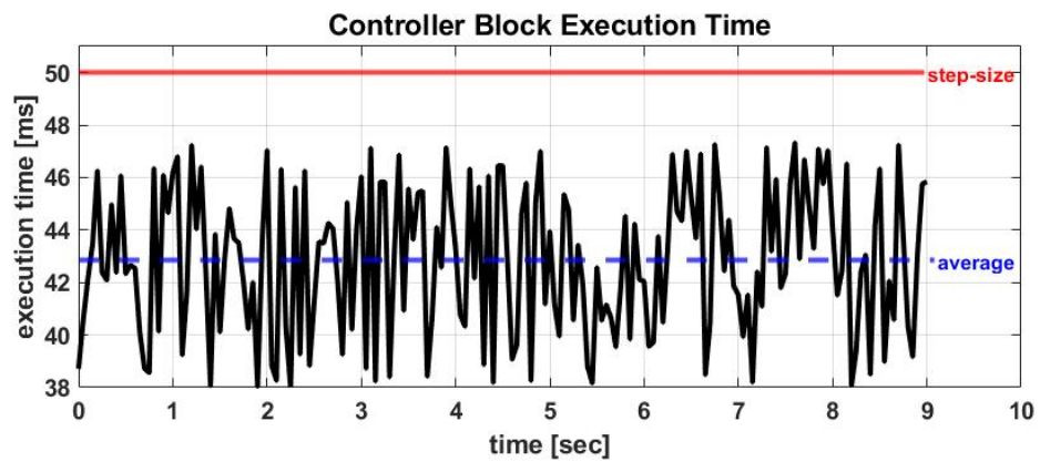
Figure 4.11: PIL Test Controller Block Execution Time
