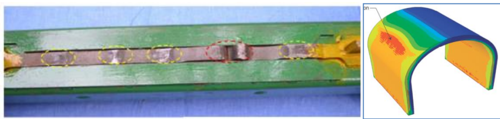
Figure 6.1 Stress concentration in (a) Core plate (b) UFP plate (Baird et al., 2014)
