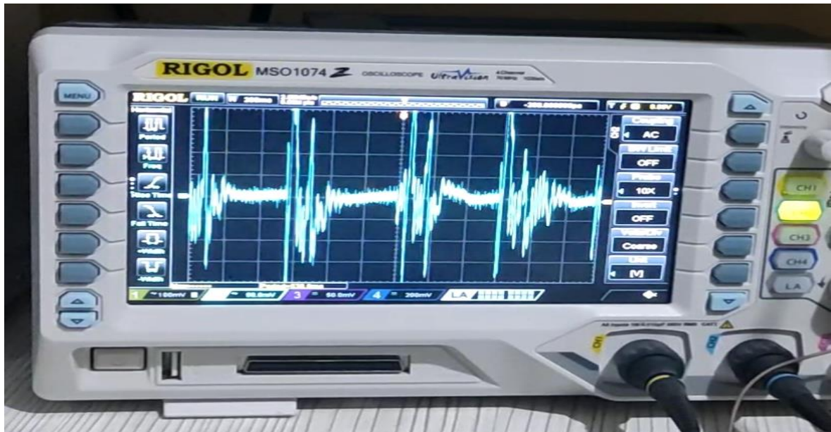
Figure 4.4. The PCG signals shown on the screen of the oscilloscope.
