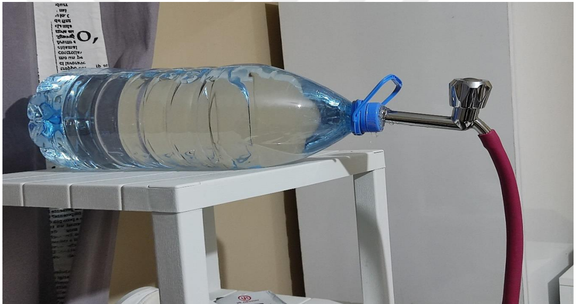
Figure 3.12. A faucet connected to 5L bottles of water.
