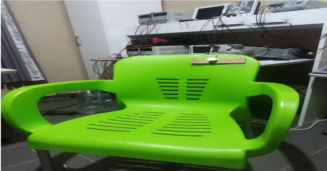
Figure 3.9. A piezoelectric transducer is placed in the inside direction of a chair.
