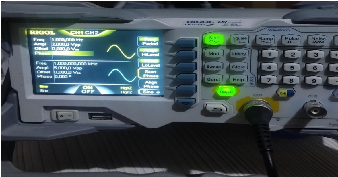
Figure 3.20. Providing the input signal from a signal generator.
