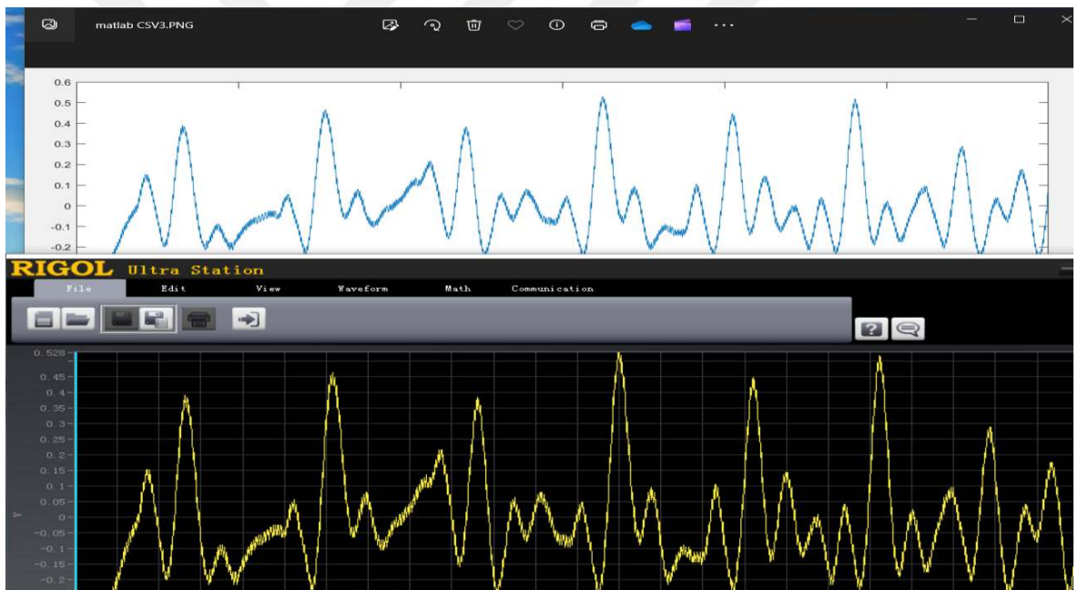
Figure 4.10. The plotted BCG signals in MATLAB and RIGOL software.
