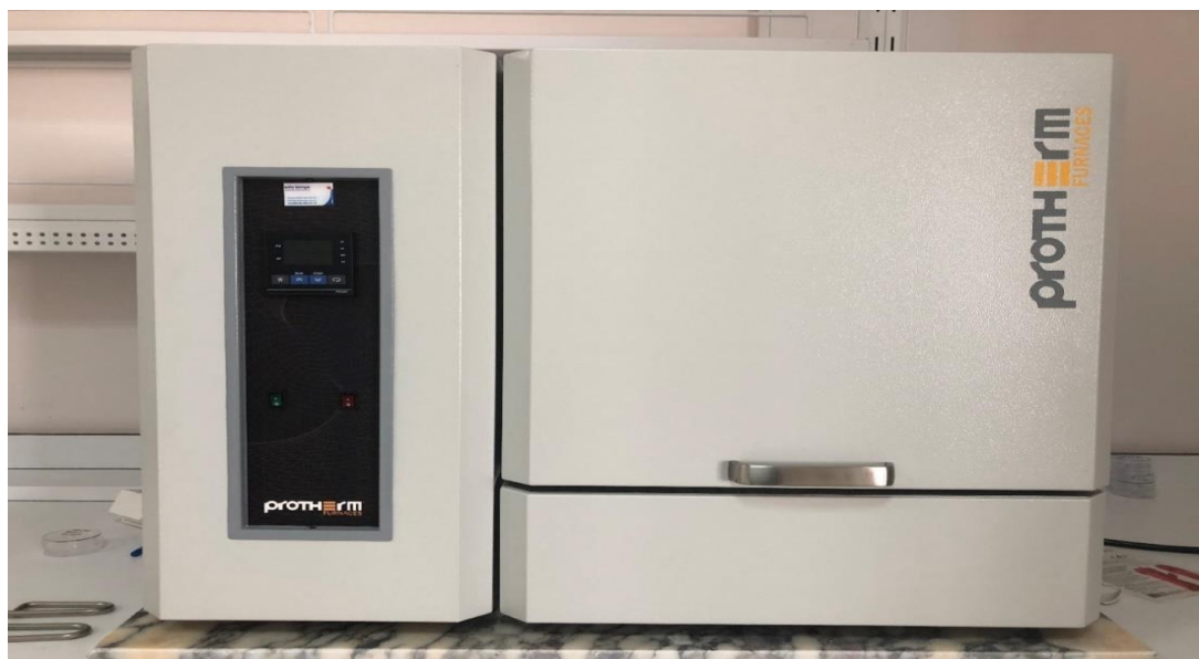
Figure 4.6. Used furnace for annealing the TNT
