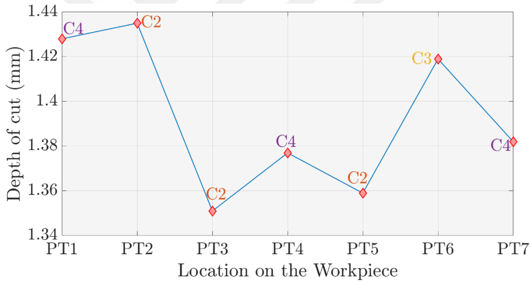
Figure 4-11: Configuration identification based on maximum stability along the tool path regarding variable spindle speed & limited configuration variation between C2—C4 in X direction
