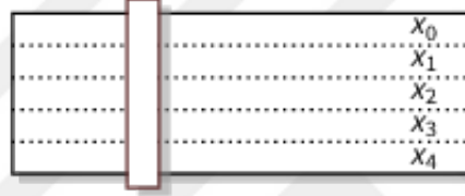
Figure 3.3: Substitution layer of Ascon. Figure was taken from the cipher's official website https://ascon.iaik.tugraz.at/images/state_vertical_small.png
