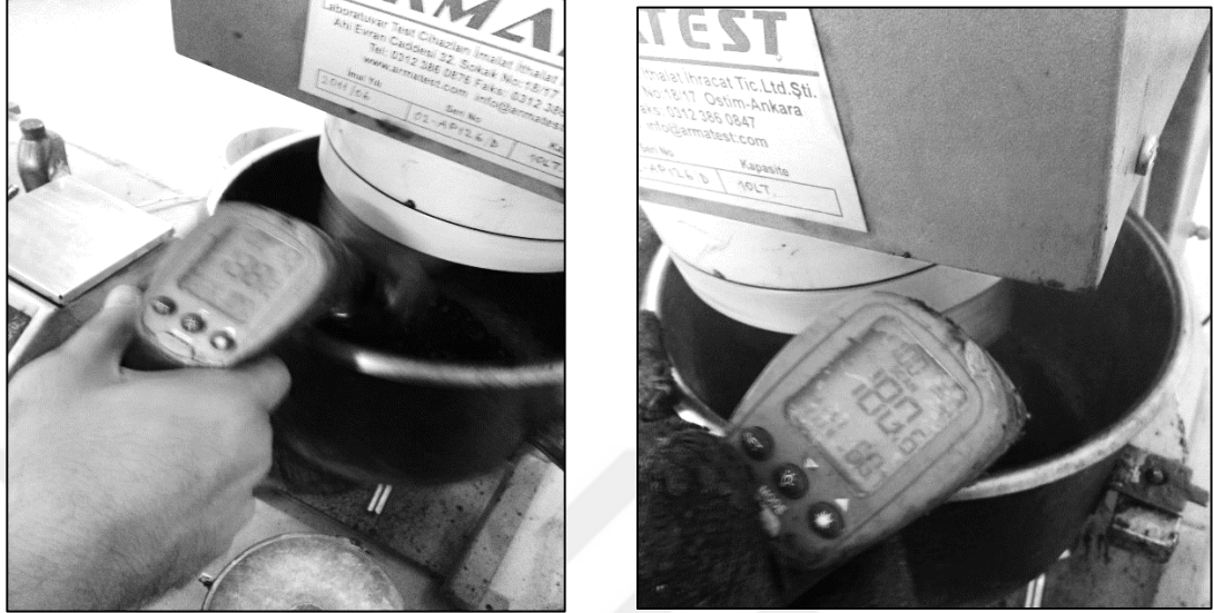
Figure 6.10 Mixing the bitumen and the aggregate at the desired temperature (Personal archive, 2019)
