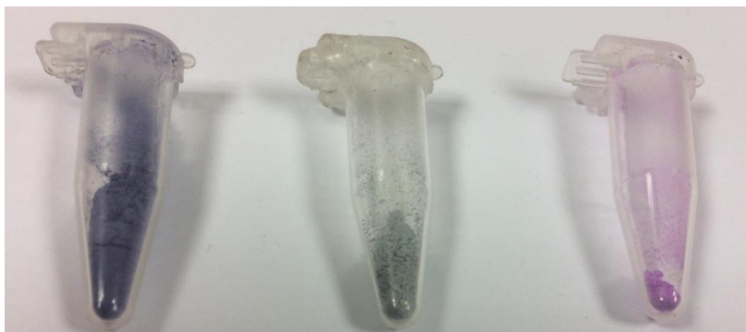
Figure 3.75. Photos of the samples calcined at 300 °C on glass, at 500 °C on glass and at 500 °C on Pyrex respectively.
