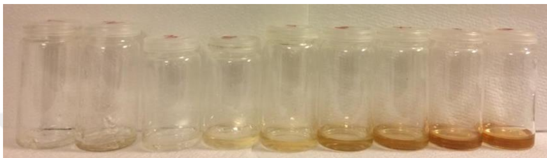
Figure 3.1. Photos of the homogeneous gels of PA-P123 in vials (from left to right, the PA/P123 mole ratio is changing from 10 to 90 by 10 increments).
