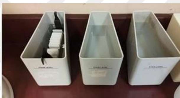
Figure 3.6: The three dewaxing tanks.
