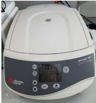
Figure 8.8. The Centrifuge (Microfuge 20R – BECKMAN COULTER)
