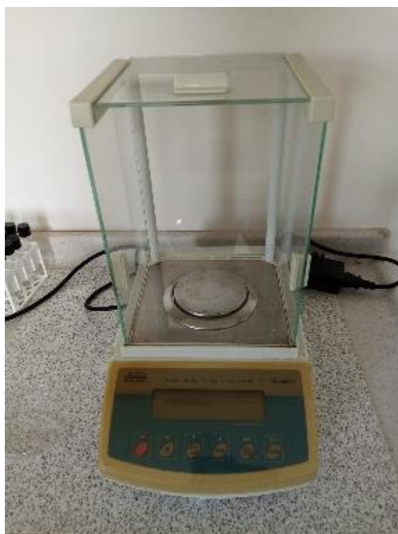
Figure 8.5. AS 220.C2 PLUS Sensitive scale
