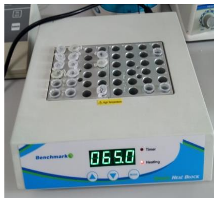
Figure 8.12. Benchmark Scientific BSH1002 Digital Dry Bath Heater
