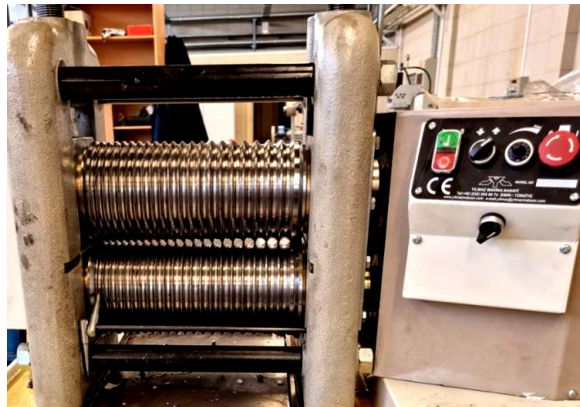
Photo 2.3. The groove rolling machine.
