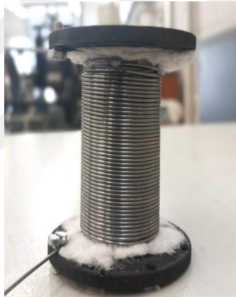
Photo 2.22. The in-reacted coil former of 3 layers of \text{MgB}_2/\text{Fe} long wires.
