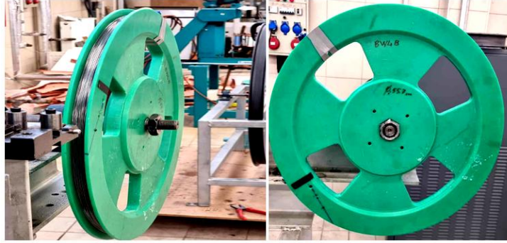
Photo 3.1. A 180-meter-long \text{MgB}_2/\text{Fe} wire of a diameter of 1.02 mm is wound around a polyethylene pulley with a diameter of 550 mm.
