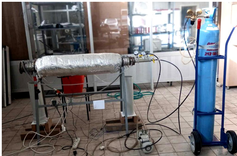
Photo 2.7. The furnace was used for sintering of wound coils with a set temperature of 680 °C.
