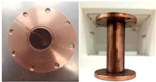
Photo 2.19. The top and vertical views for the copper former.
