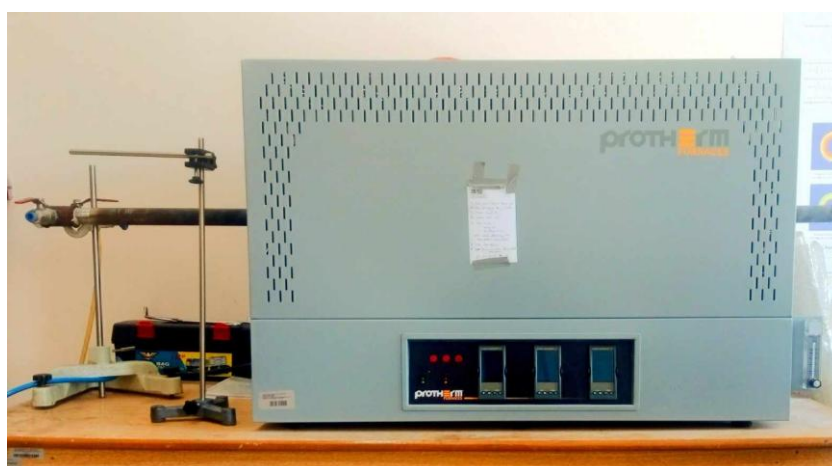
Photo 2.6. Three Zone Programmable Furnace.
