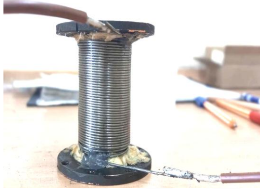
Photo 2.23. The reacted coil of 3 layers after heat treatment process.
