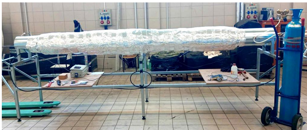
Photo 2.8. The 4m long tube furnace used for continuous heat treatment.
