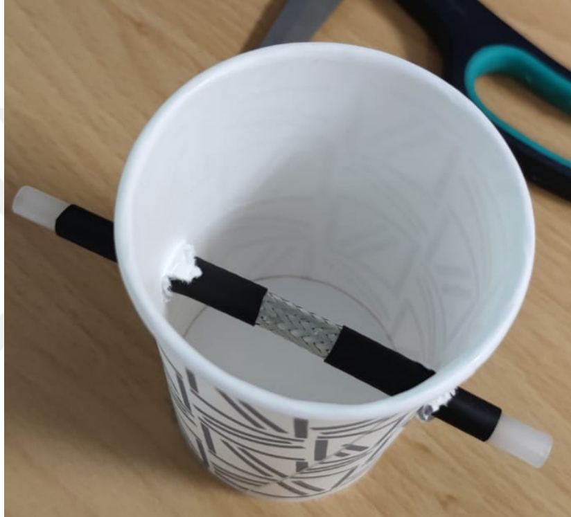
Figure 31: The leaky pipe and box for tests.
