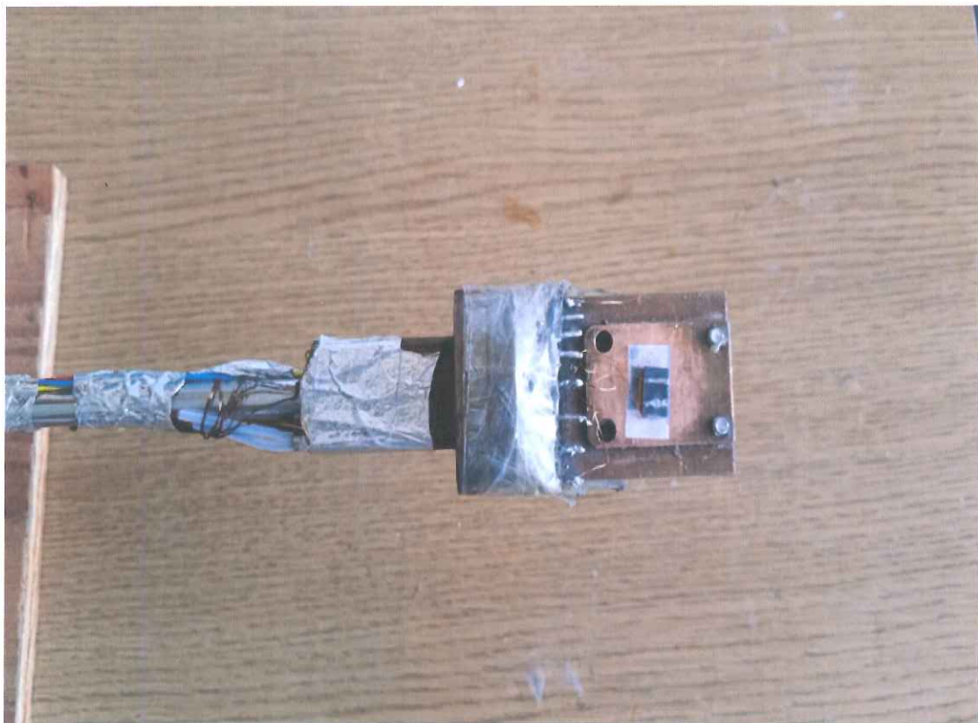
Figure 3.7. Experimental set-up for the 4-point probe measurement.
