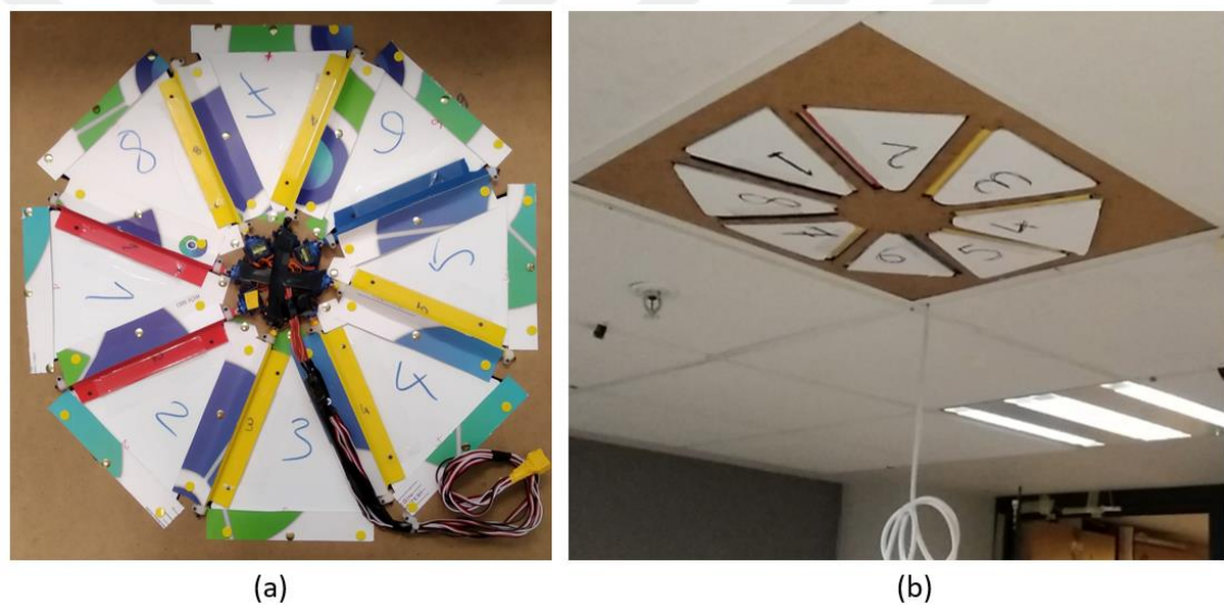
Figure 20: Pictures of operable-flap diffuser prototype: (a) back side (b) on the ceiling as mounted.
