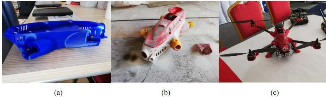
Figure 6.4: (a) Produced quadcopter structure, (b) during post-processing, (c) Final state of quadcopter.
