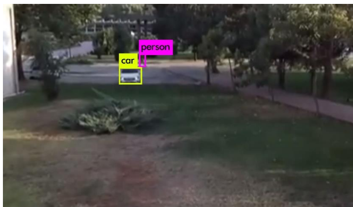
Figure 7.4: (c) Generated new model of YOLOv3 on more data and with more iteration has successfully detected both the person and the car at 0.5 IoU.
