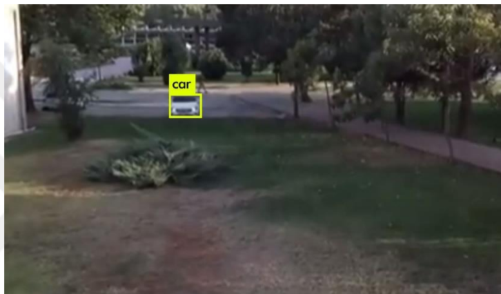
Figure 7.4: (b) Default YOLOv3 model has detected only the car, but not the person.
