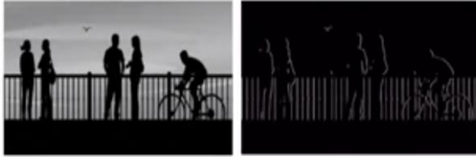
Figure 3.13: (a) Input image for vertical edge detection. (b) Vertical edges are detected with convolution operation [21].
