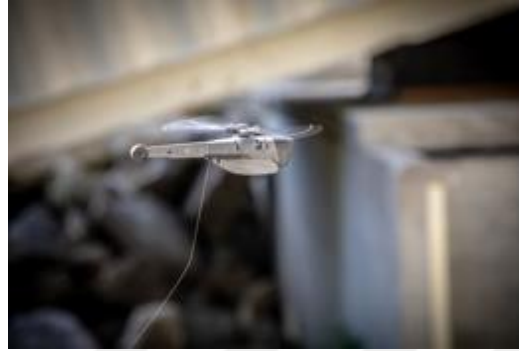
Figure 1.2 Black Hornet Micro UAV
