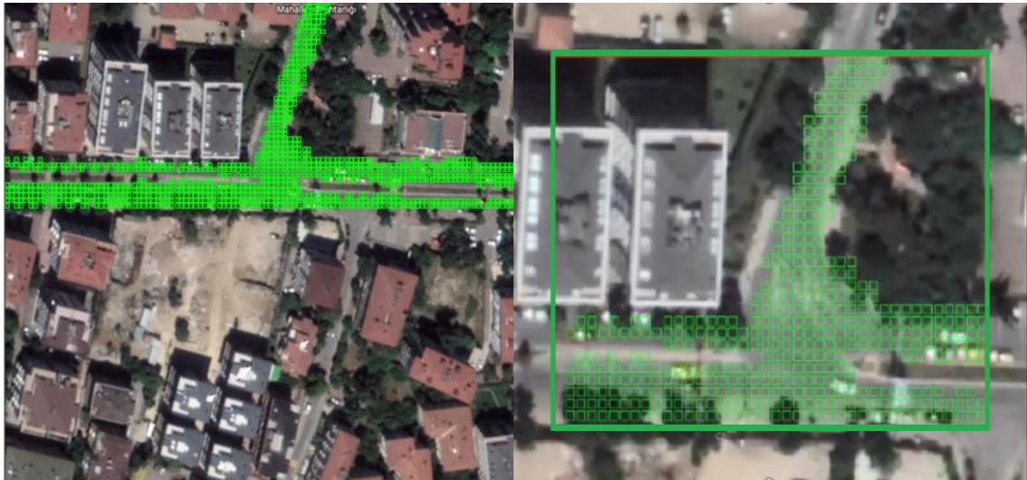
Figure 6.5. Visualization of occupancy map and workspace of the construction site
