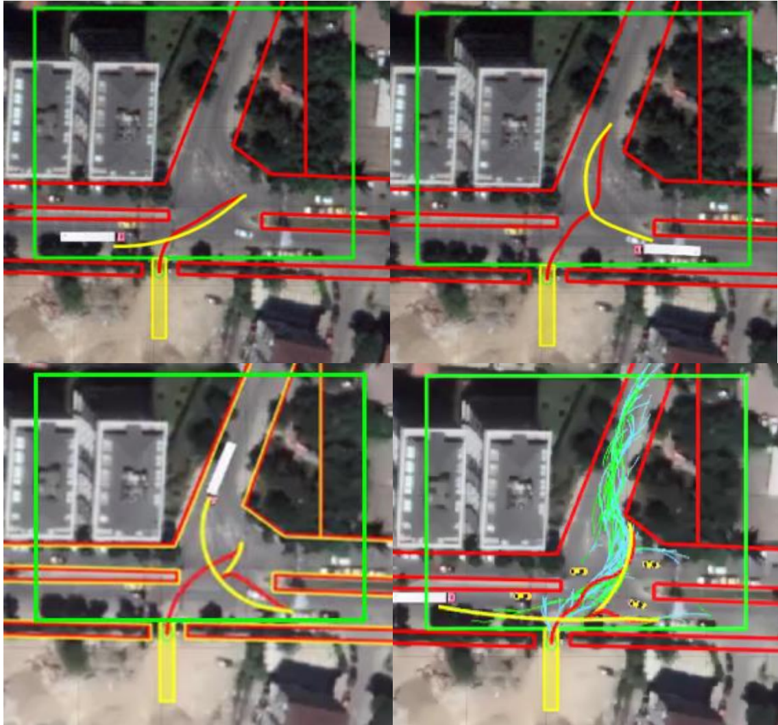
Figure 6.6. Resulting parking paths for different scenarios on construction site
