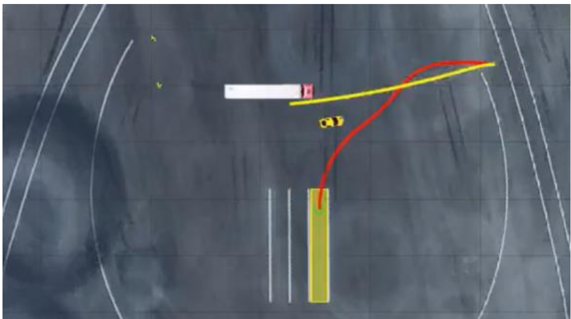
Figure 6.1. Resulting parking path for scenario 1
