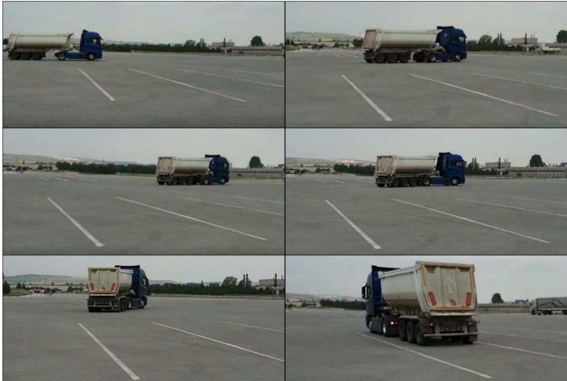
Figure 6.28. Real-world visualization of autonomous trailer parking maneuvers with fully equipped Ford F-MAX truck at Inonu test facility
