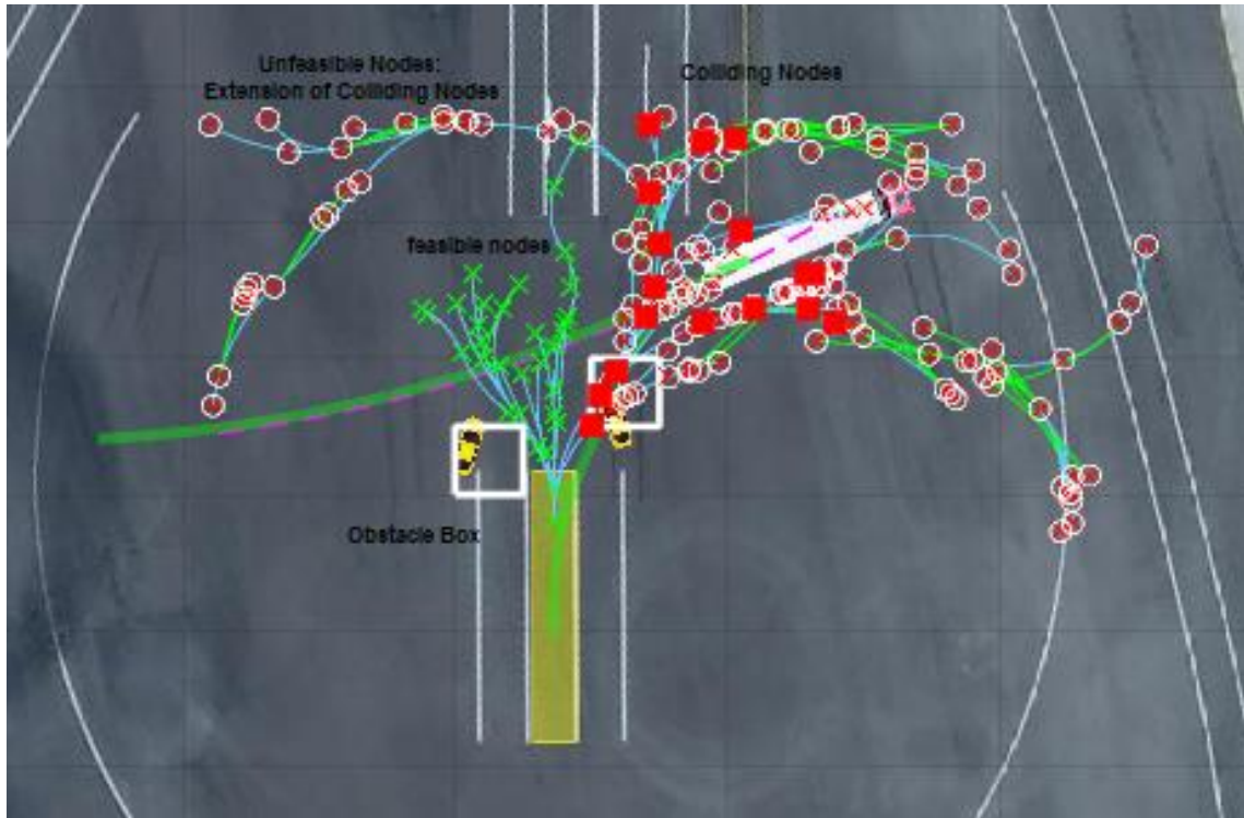
Figure 4.10: Updating Tree by deleting unfeasible nodes
