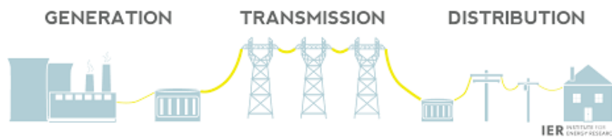
Figure 1.1: Electricity Generation, Transmission and Distribution (source: www.instituteforenergyresearch.org )
