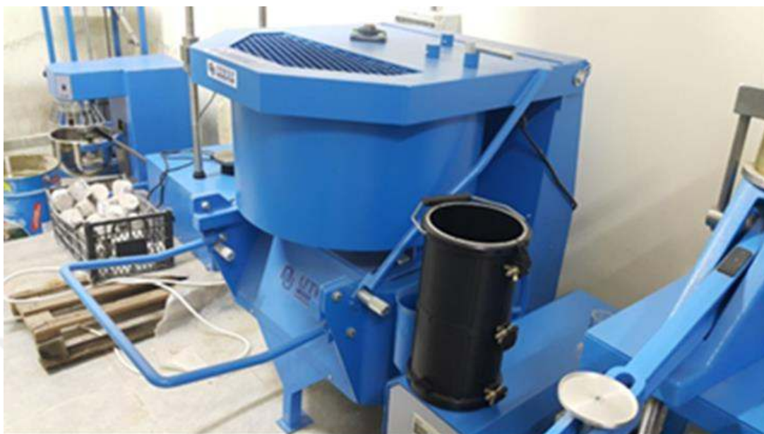
Picture 3.2 Concrete mixer and cylindrical mold
