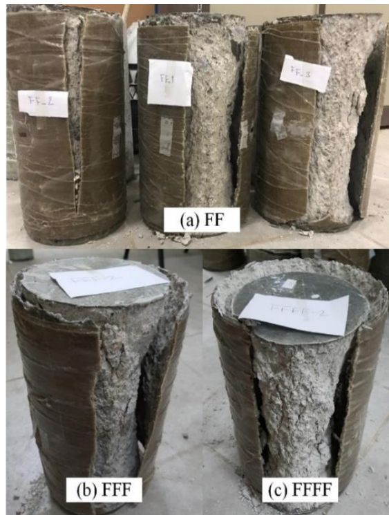
Picture 4.4 Failure mode for FFRP groups
