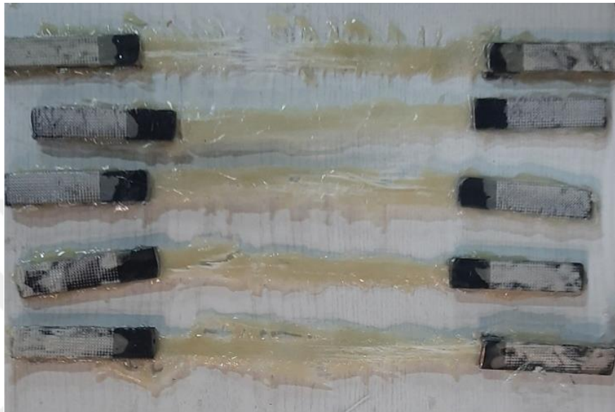
Picture 4.2 Failure mode of GFRP
