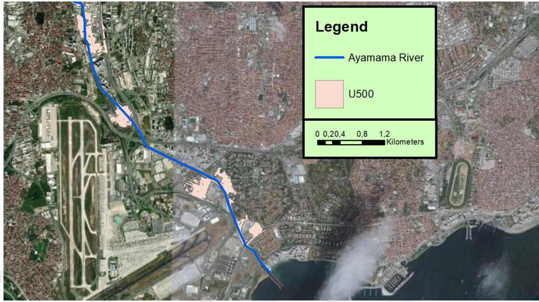
Figure 4-4 Flood inundation with 500 year return period flow in the Ayamama River (Downstream)
