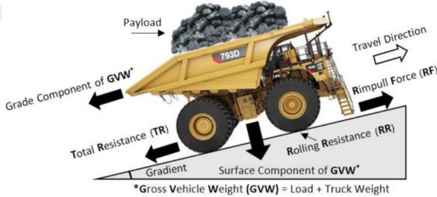
Figure 3.2. Body Diagram of Truck (Soofastaei et al. , 2016)
