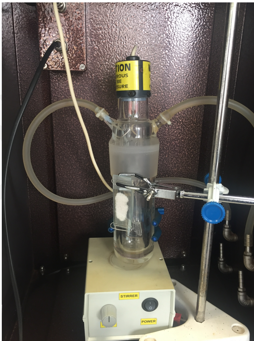
Figure 12. The appearance of the reaction set-up before the UV lamp is switched on.
