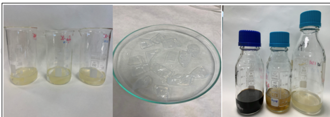
Figure A.1. Experimental set-up a) bacterial cellulose pellicle was treated with 2M NaOH at 80°C for 1h b) bacterial cellulose pellicle was broken into pieces c) sulphuric acid pretreatment with autoclave (90% sulphuric acid left; 65% sulphuric acid middle; 40% sulphuric acid left)
