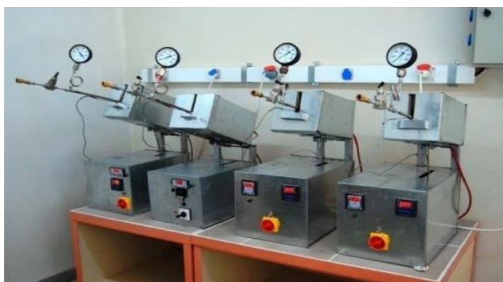
Figure 4.2.1.2 Schematic view of batch autoclaves and their auxiliaries.
