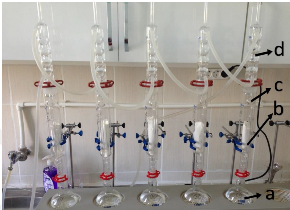
Figure 3.1. Soxhlet apparatus a) Distillation flask, b) Sample, c) Thimble-holder, d) Where solvent is chilled.
