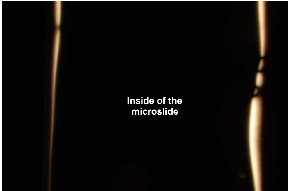
Figure 14. The pseudo-isotropic texture (extinct area) of the nematic phase. The white areas at the sides of the microslide are not yet aligned sections of the phase.
