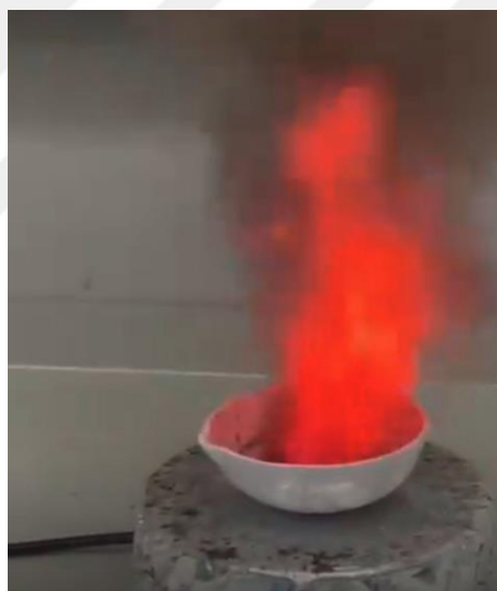
Picture 2: Solution combustion synthesis of \text{CoMn}_2\text{O}_4 with Glycine fuel
