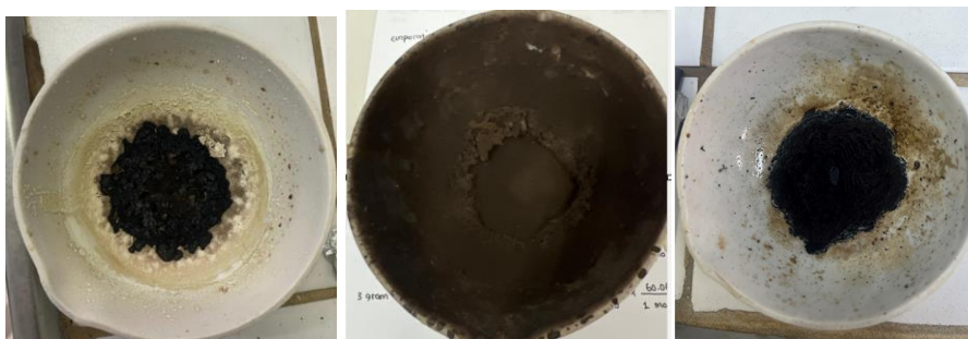
Picture 1: \text{MgMn}_2\text{O}_4 product by using tartaric acid (a), glycine (b), urea (c) fuel
