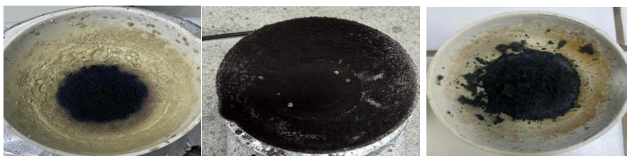
Picture 3: \text{NiMn}_2\text{O}_4 product by using tartaric acid (a), glycine (b), urea (c)
